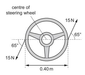
Each force has a magnitude of 15 N and acts in the direction shown. The steering wheel has a diameter of 0.40 m.
