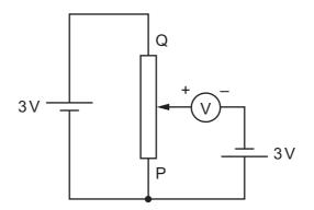
The sliding contact is moved to end P of the potentiometer and then to end Q.
