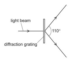
The diagram shows only the **second**-order maxima that are produced.
