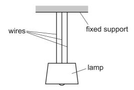
The weight of the lamp causes each wire to have an extension of  $0.40\,\mathrm{cm}$ . The height h of the lamp above the floor is measured.
