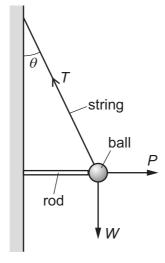
The string is at an angle  $\theta$  to the vertical. The tension in the string is T. The ball is held away from the wall by a horizontal force P from a metal rod.
